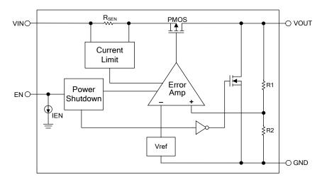
Figure 3. Block Diagram of FP6168
