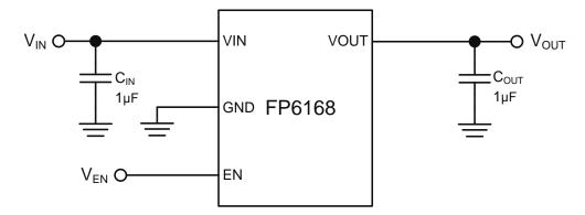
Figure 2. Typical Application Circuit of FP6168
